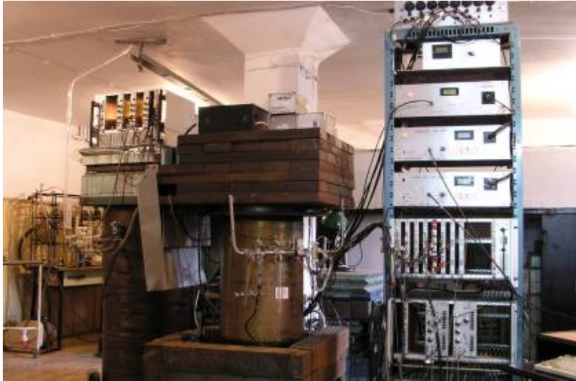
Fig. 4 Site of 5 gas proportional counters (L1, L3, L4, L5 and L6) in Gliwice Radiocarbon Laboratory: in the front – L1, L3 – behind of L1 on the right, L4, L5 and L6 counters in iron shield on the left of L1).
