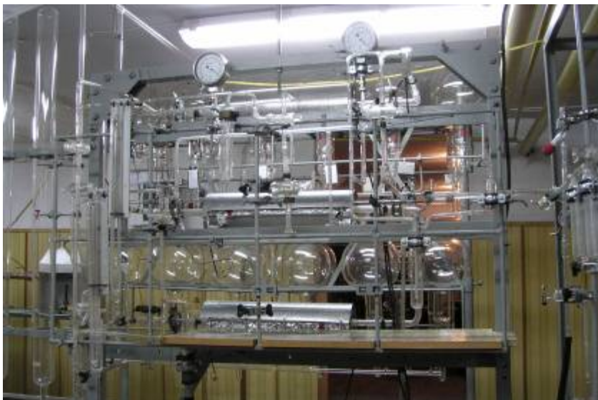
Fig. 3 Fragment of vacuum line with ovens containing Ag and Cu (500°C) and water traps, used for purification of CO 2 and for filling gas proportional counters.
