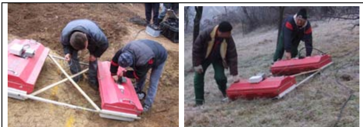
figure 2: radar antenna 100 kHz
