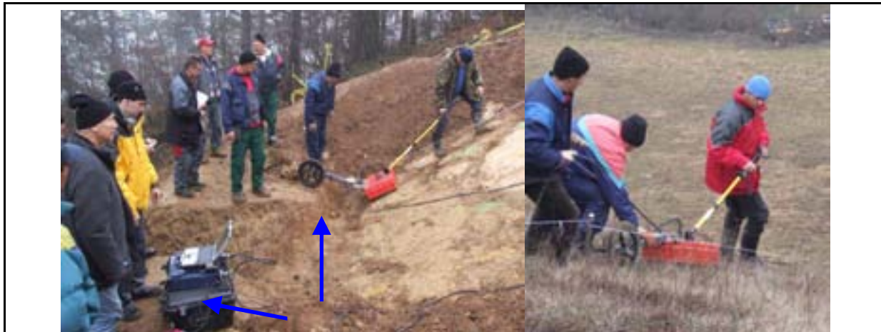
figure 1: radar equipment left: computer, middle and right: radar antenna 270 kHz
